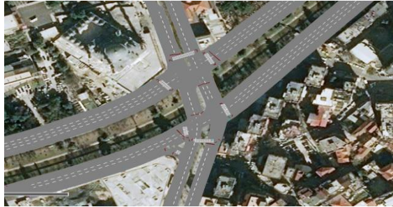
Fig. 2. Construction of two intersections in VISSIM
